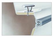
1985 Innovation of the energy-efficient sandwich hull and Divinycell application.
