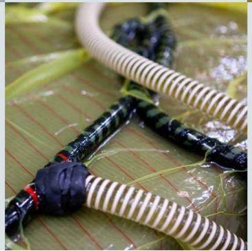
The unique properties of the vacuum infusion method combined with high quality materials, ensure high rigidity, strength and minimum weight. Above: a complete set of precision cut, multiaxial glass-fibre matting.
